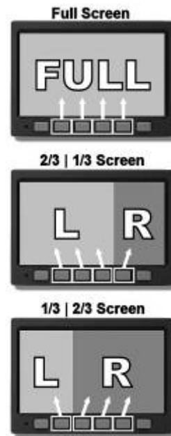
Figure 6 - The configuration of the pages on the screen determines which buttons are used to display a page's menu.
