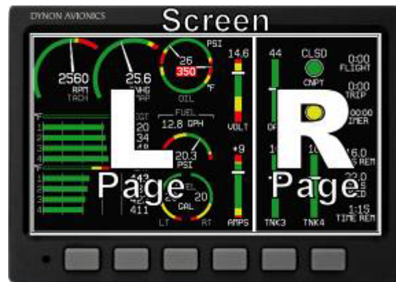
Figure 2 – Screens contain one or two pages and pages contain groups of similar information.
