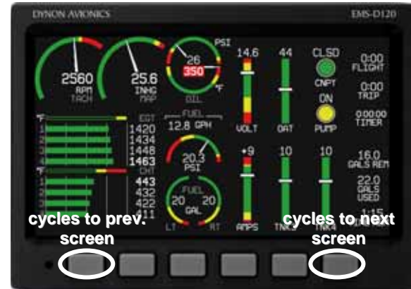
Figure 5 –Buttons one and six cycle to the previous and next screens, respectively.
